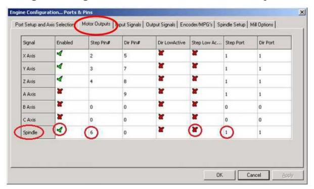
2. Engine Configuration... Ports & Pins – Spindle Setup
