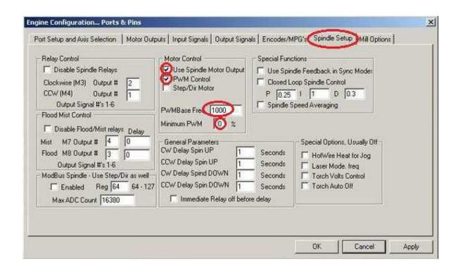
**IMPORTANT!** You need to set PWM Base Freq between 5 000 and 10 000 Hz. Setting lower frequency value (e.g. 1000 Hz, 10% duty) is incorrect because laser is turned on at maximum power only by 0,1 milisecond and turned off by 0,9 milisecond. As a result, power of laser isn't averaged and cutting (engraving) line is dotted with long pauses especially if engraving speed is high.
