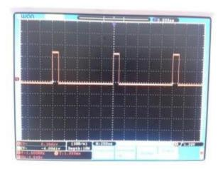
If you set higher base frequency, for example 10 000 Hz and the same duty, laser is turned on at maximum power 10 times per 1 milisecond. As a result, power of laser **is averaged** and cutting (engraving) line is homogenous.
