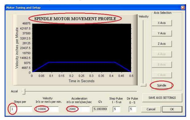
You can connect pin number 6 of the breakout board (or another, if you set them) directly to the TTL input of the laser head. After these, you can enter a spindle speed between 500 and 10.000 and Mach will control the laser as a spindle. The spindle speed will adjust the laser power.
